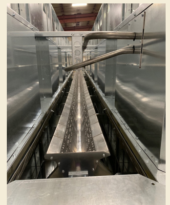
Burner with internal vaporizer
